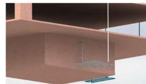
After cooling the building, the water gets heated. This heated water is then carried through a pipe to the UWR. On the way to UWR the heated water is again cooled with geothermal effect.
